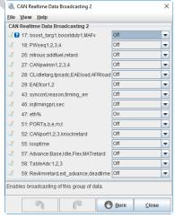
default value (1520). Then set a "Broadcasting rate" to 10 Hz. Then, click on "CAN bus/Test modes" again and select "CAN Realtime Data Broadcasting 2". Set value "47:eth%" to ON.
